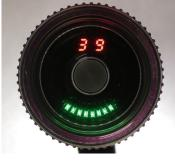
The charge level monitor circuit shows the available energy by taking into account charge and discharge currents.
