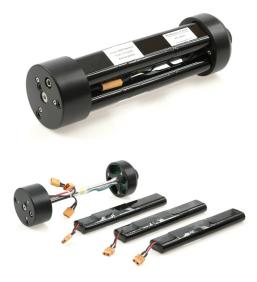
IMPORTANT: The total capacity of the battery pack exceeds the maximum capacity for Li-Ion battery allowed on airplanes! Therefore the battery need to be disassembled for safe transport on airplanes. After disassembling you can carry safely three single batterypacks, each one will be below the maximum capacity limit.
